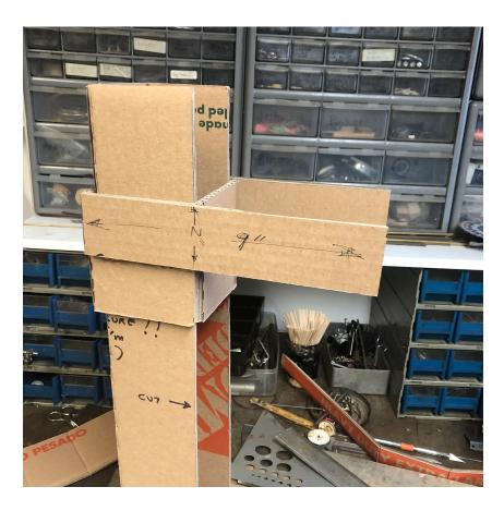
11. In the following steps you'll be making the camera mount. Some of the your measurements will be determined by the design of your camera. I'm using a small Motorola camera as an example (I'm using my iPhone to shoot this and the Motorola is from a few years back). Measure out a piece of cardboard to fit flush between the two pieces for the support. Do Not glue it in place yet!
