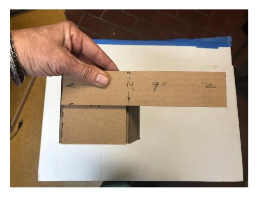
10. Glue these in place, one on each side and slip the sleeve back onto the tube.
