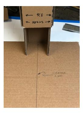
7. Draw a center line on the base and use this to center the vertical tube. Draw around the base of the tube to mark the slots where the tube locks into the base. In the photo on the right I've cut out the slots.
